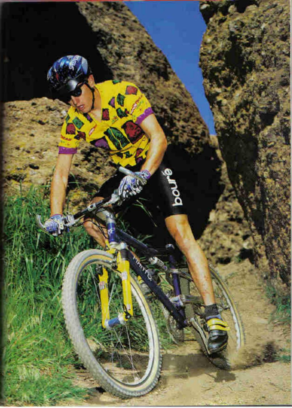
The Mantis Pro Floater was one of the first MacPherson Strut full-suspension designs to hit the mountain bike scene. From the beginning, the Mantis Pro Floater was well-received by cross-country riders. Like all early MacPherson Strut rear-suspension systems, the Pro Floater suffered in two performance
