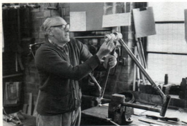
Figure 8-2: Ken Taylor fits the bottom bracket on a custom tandem.
