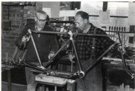
Figure B-1: Ken (left) and Norman Taylor inspect a newly brazed tandem frame.
