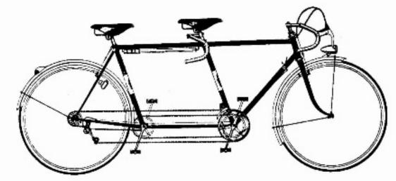
FRAME. 22"-21" with sloping top tube or to order. Open design as illustrated or double diamond. Built throughout from Reynolds 531 tubing and Bronze welded construction. 73-71-69 degs. 63" wheelbase, 11" Bracket height, 2½" Rake oval section forks. All brazed parts for gears, brakes,
