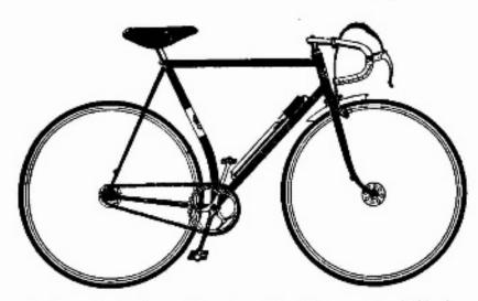
A short wheelbase machine of special design, most suitable for hill climbs and short distance time Trials. Weight, as illustrated, 193 lbs.
