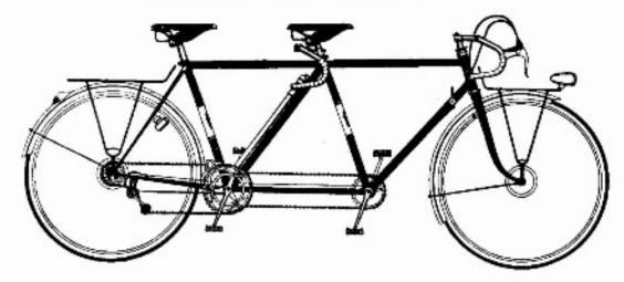
FRAME. Sizes to order with parellel or sloping top tube Double Diamond Design. 63" wheelbase, 11" Bracket Height, 29" rake oval section forks. Brazed on parts for all fitments.
